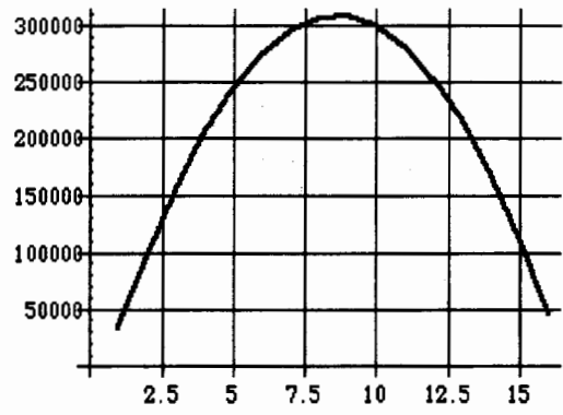
Fig. 5b. Magnetic field distribution on the measured surface
