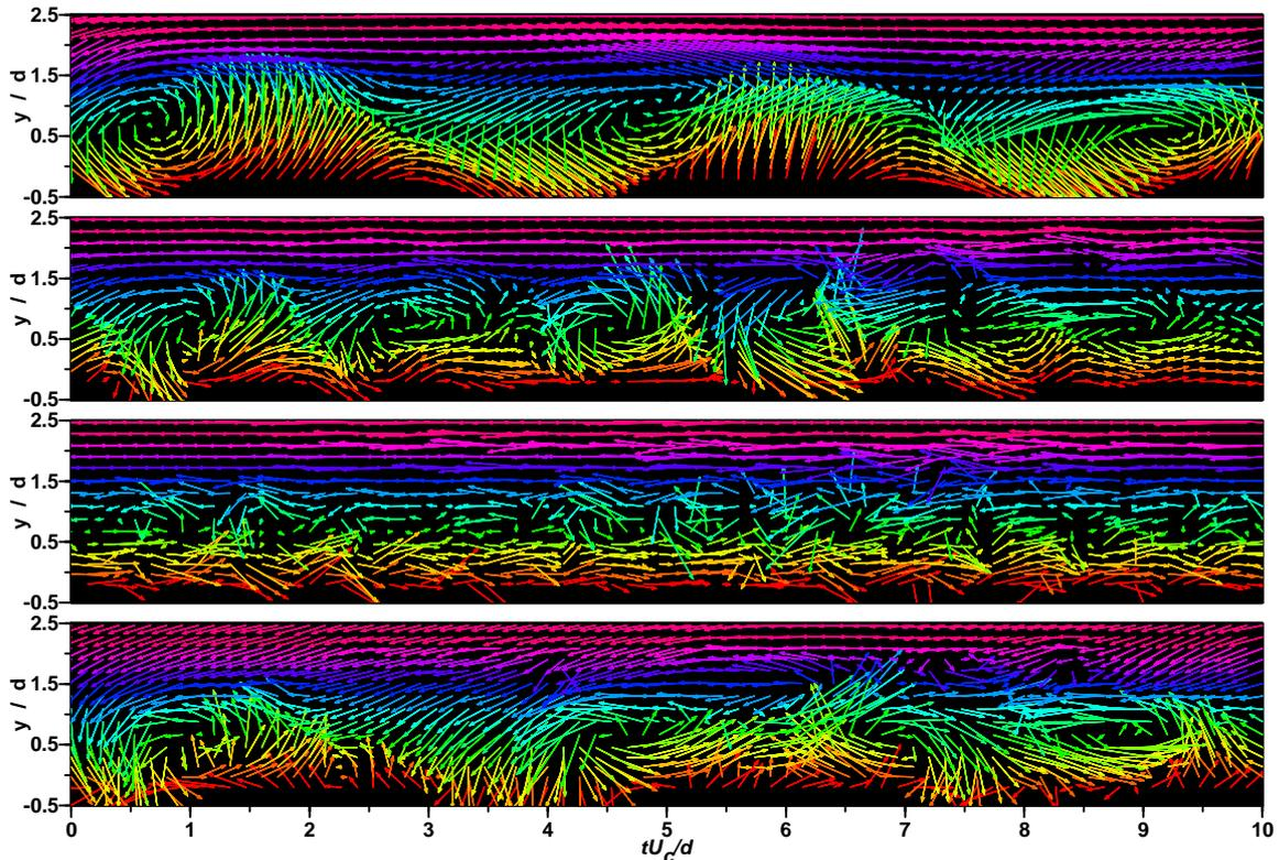
Figure 2 Multiresolution velocity vectors of wake flow
