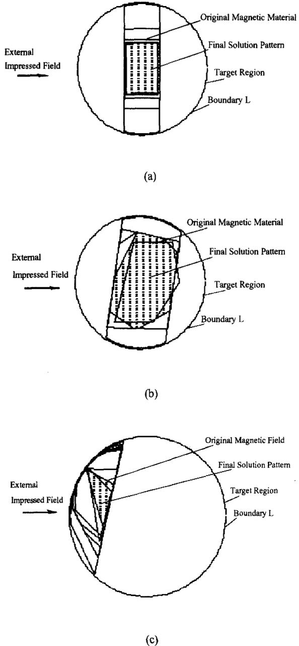
Fig. 1. Shape and location identification of magnetic material with different cross section shape. (a) Magnetic material with rectangular cross section shape. (b) Magnetic material with polygonal cross shape. (c) Magnetic material with triangular section shape.
