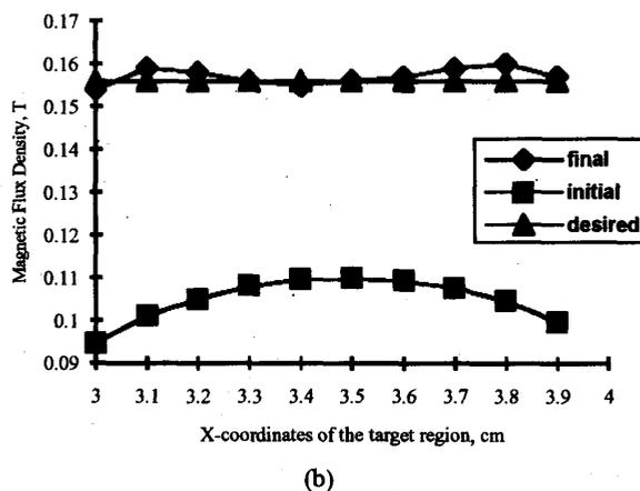
Fig. 2. Pole design of magnetic core. (a) The initial shape of the pole and final solution pattern. (b) Distribution of magnetic flux density at initial and final shape of poles.
