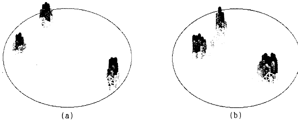
Fig.3 Improved plural defect recognition. (a) Improvement by shrinking the target area, (b) improvement by removing the pilot points up to the first peak.
