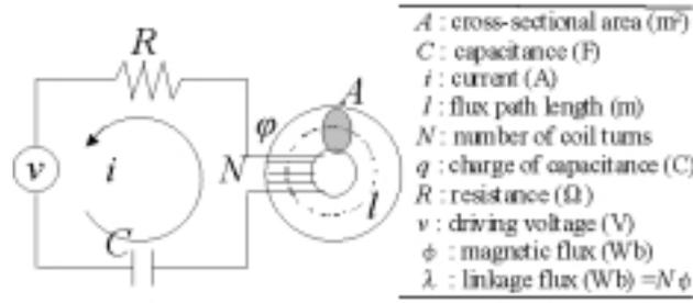
Fig. 2. Series ferroresonant circuit.
