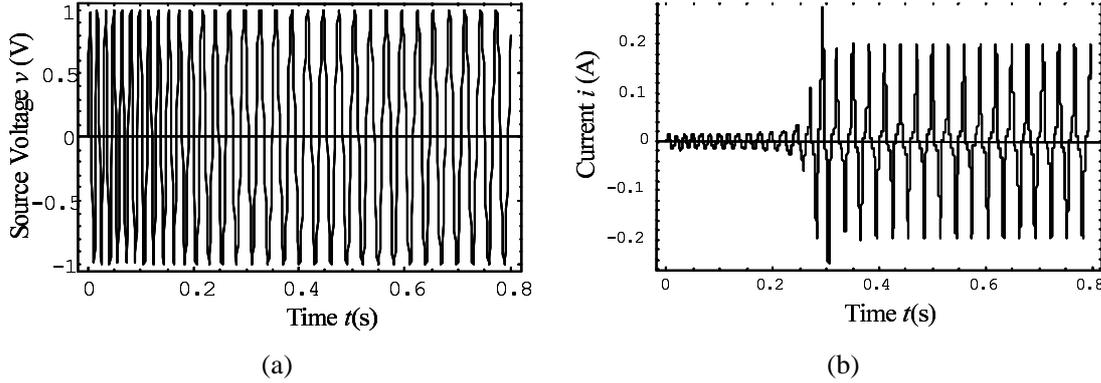
Fig. 3. Ferroresonant phenomenon. (a) Driving voltage  $v$  vs. time  $t$ . (b) Current  $i$  vs time  $t$ .
