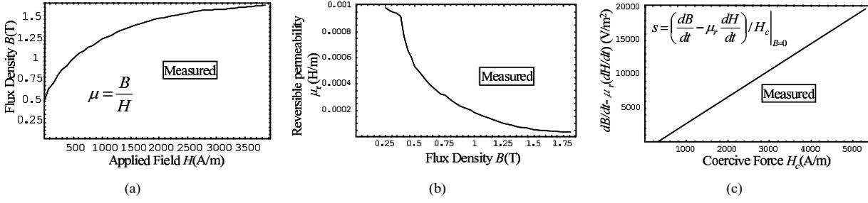
Fig. 1. Parameters of Chua-type magnetization model (Measured: soft iron). (a) Permeability  $\mu$ . (b) Reversible permeability  $\mu_r$ . (c) Hysteresis parameter  $s$ .
