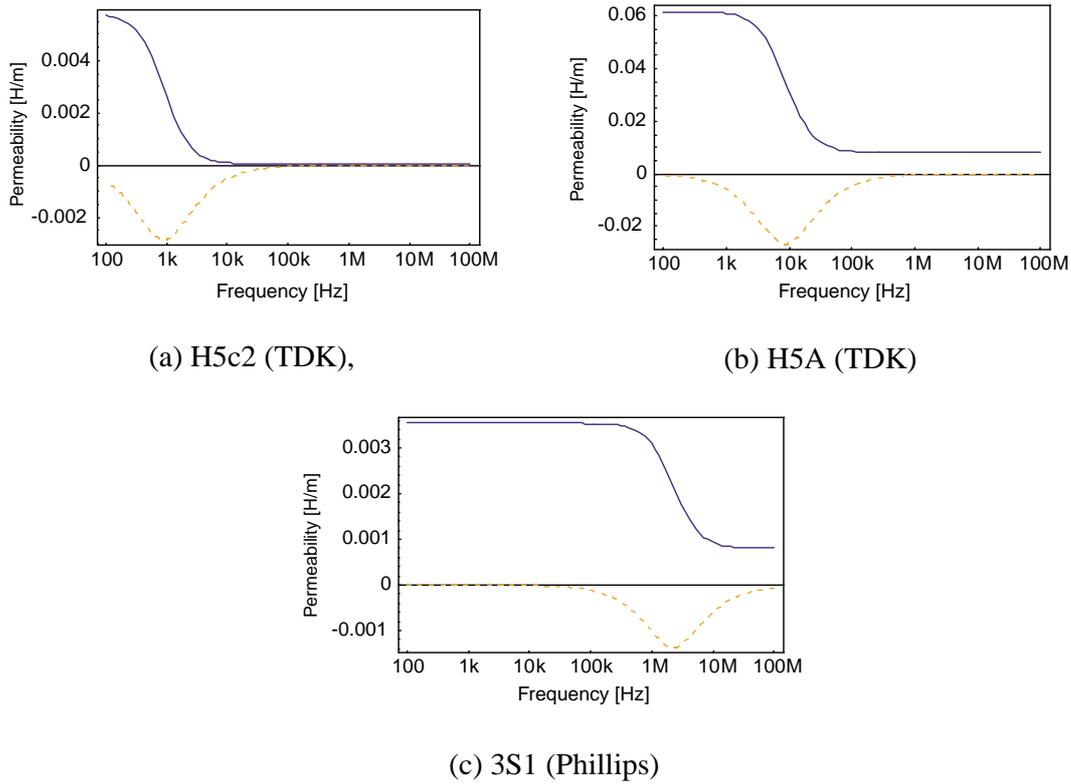
Fig. 3. Frequency characteristics of the complex permeabilities (solid line : Real part, broken line : Imaginary part).
