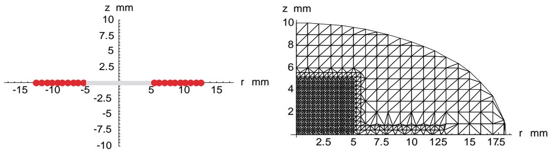
Fig. 2. Schematic diagram of a planar inductor and mesh system for FEM analysis.
