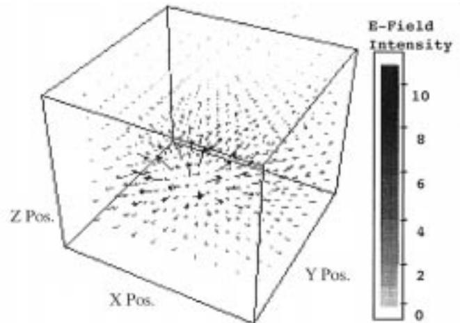
Fig. 7. Three dimensional electric field vector distributions.
