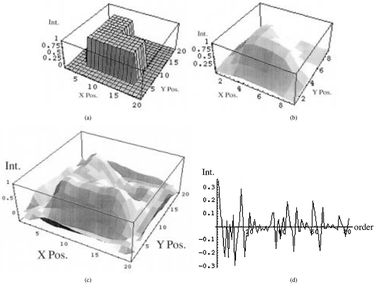
Fig. 4. (a) Model Source distribution; (b) Measured field intensity; (c) weighted inverse solution and (d) the coefficients of Fourier series.
