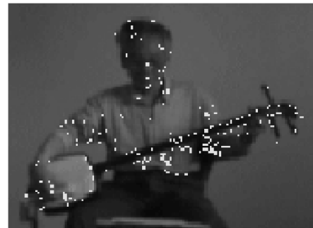
Fig. 8 1/f Fluctuation Frequency Extraction from a Music Instrument (Shyamisen) playing White dots denote the 1/f fluctuating pixel position.
