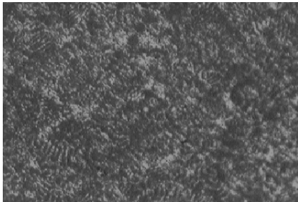
Fig. 9 A Magnetic Domain Image by Bitter Method Sample: soft iron
