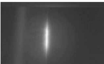
Fig. 6 Infrared image of two iron plates when simulating a crack by connecting two iron plates
