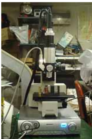
Fig.9 Experimental device for magnetic wall observation.
