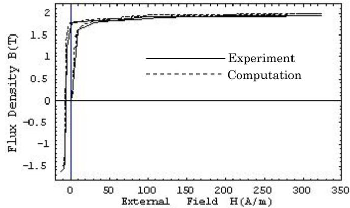
Fig. 5. Magnetization Curve Reconstruction Based on (3)
