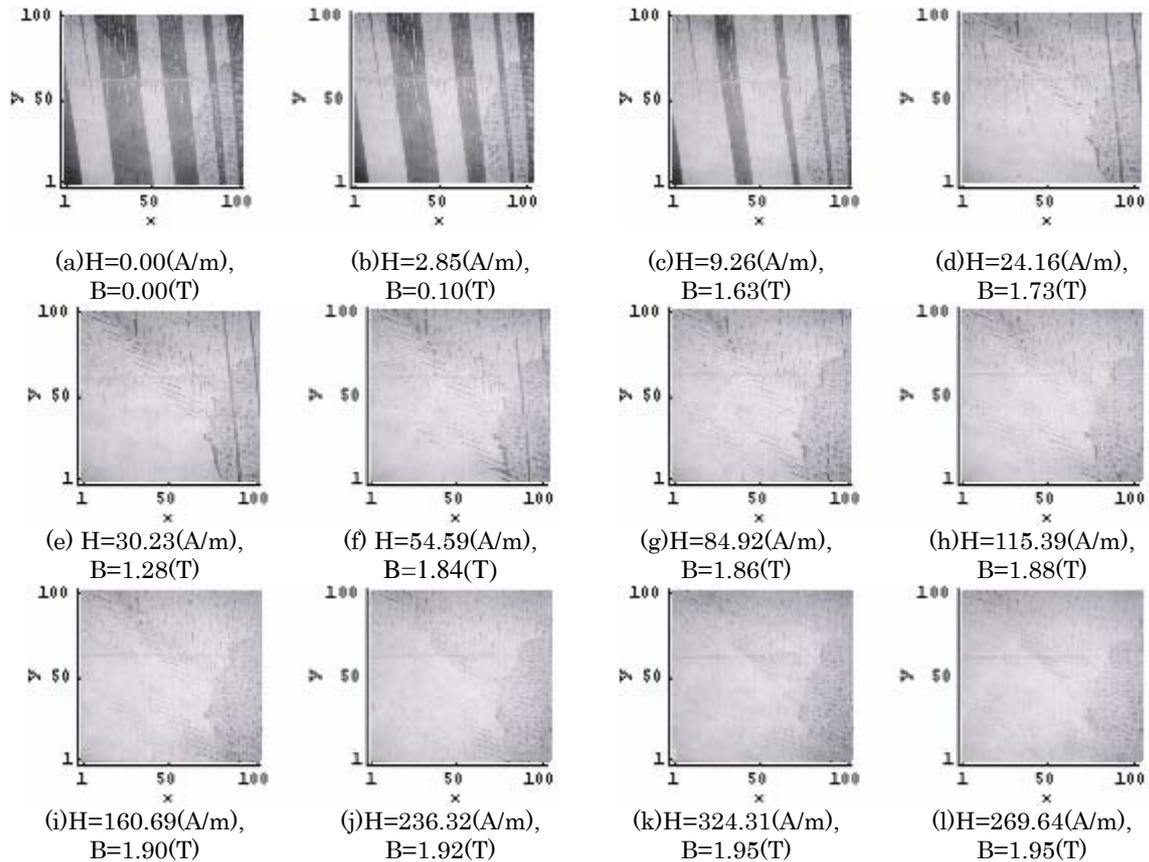
Fig. 1 Examples of Magnetic Domain SEM Images (100x100 pixels, 0.1 mm/pixel)
