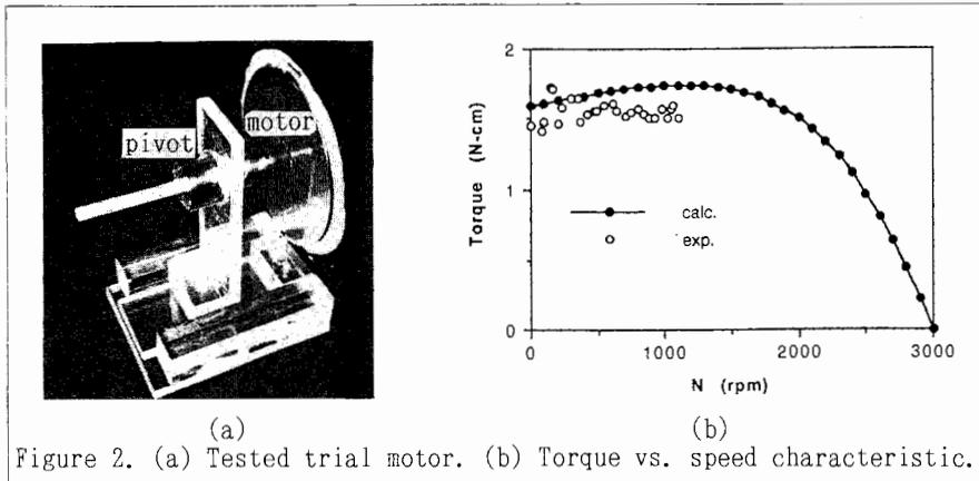
Figure 2. (a) Tested trial motor. (b) Torque vs. speed characteristic.
