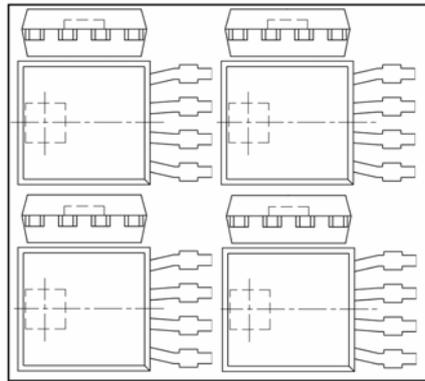
Figure 14. X-Y magnetic field flux density components array.
