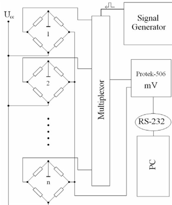
Fig.16. Signal pick-up circuit with Protek506.
