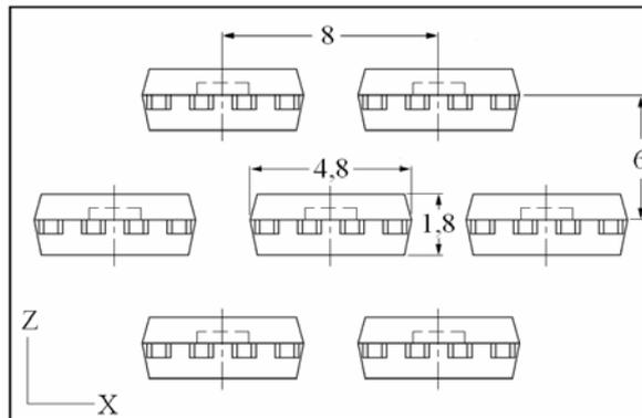
Fig.13. 7-element hexagonal array.
