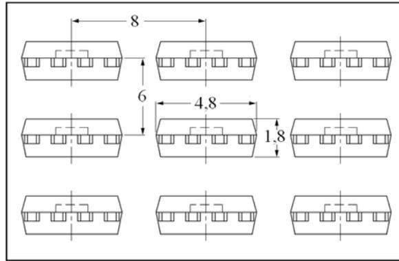
Fig.12. 3x3-element square array.
