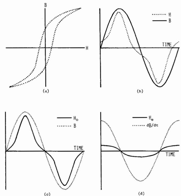
Fig. 1. (a)  $B$ - $H$  loop; (b) time variations of  $B$  and  $H$ ; (c)  $B$  and odd component  $H_o$  of  $H$ ; and (d)  $dB/dt$  and even component  $H_e$  of  $H$ .
