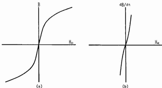
Fig. 2. (a)  $B-H_o$  curve which represents the saturation property; and (b)  $dB/dt-H_e$  curve which represents the hysteretic property.
