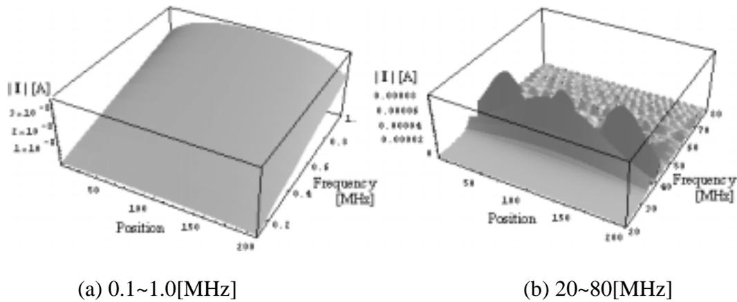
Fig. 7. Displacement current distribution vs. frequency characteristics.
