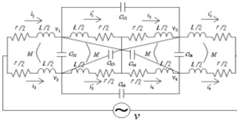
Fig. 3. Equivalent circuit of a film conductor where  $m = 4$ .
