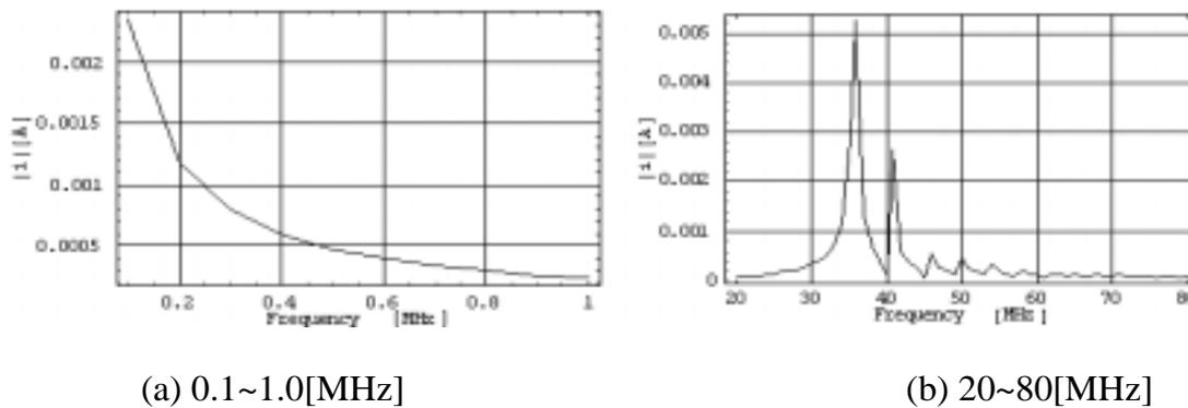
Fig. 4. Entire current  $i$  vs. frequency characteristics.
