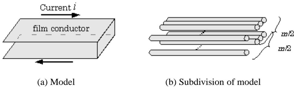
Fig. 1. Semi-analytical modeling of a film conductor.
