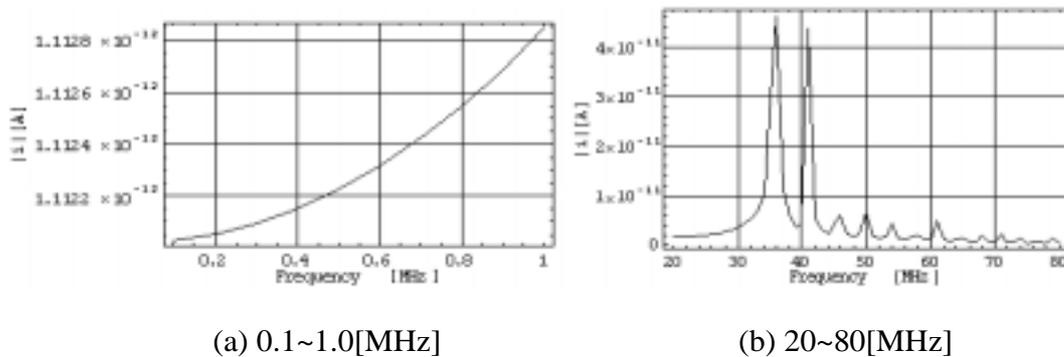
Fig. 6. Displacement current vs. frequency characteristics.
