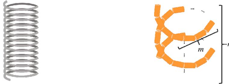
(a) Original finite length solenoid inductor. (b) Modeling of finite length solenoid inductor.
