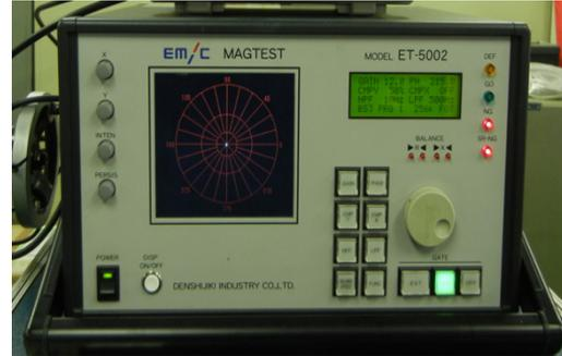
**Fig. 6. Japanese standard ECT signal processor "ET-5002" made by Emic (Denshijiki Industry) Co., Ltd.**
