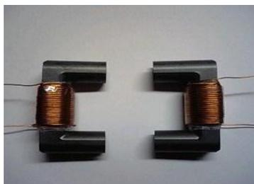
Fig.1 U shape ferrite core transformer
