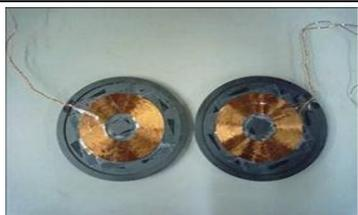
Fig.2 Soup plate like ferrite core transformer
